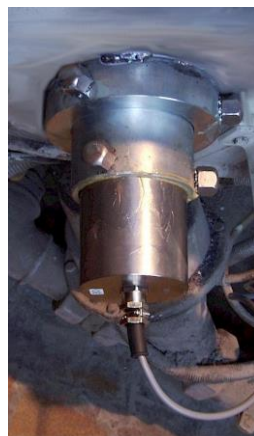
Installation of a mixer probe in the bottom of a pan mixer using a wear protection tile.
